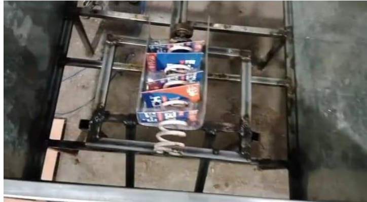
Figure 2 Fabricated model of smart medical vending machine
